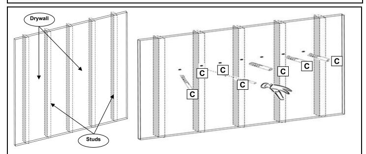
**STEP 2. A.** Locate the wall studs using an electronic stud-finder. Mark the hole locations with a pencil. The holes should be 8" (20.3 cm) apart, and level. The minimum height from the surface below must be 6" (30 cm). **B.** Three screws should be screwed directly into wall studs. Then, four drywall anchors are needed.
