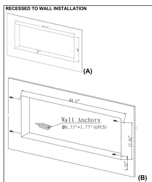
STEP A. Selection a dry wall to open a hole for fireplace box. Size of hole as below chart Figure ( A )
