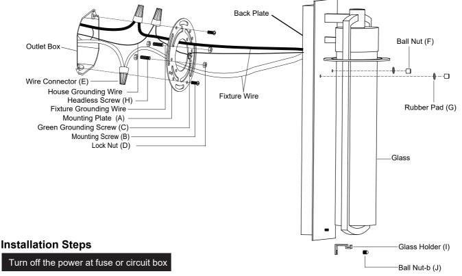
1. Thread two headless screws (H) through the mounting plate (A), then secure them with four lock nuts (D) ( two on each side of the mounting plate (A) ). Adjust the length of the headless screws (H) if necessary ).
