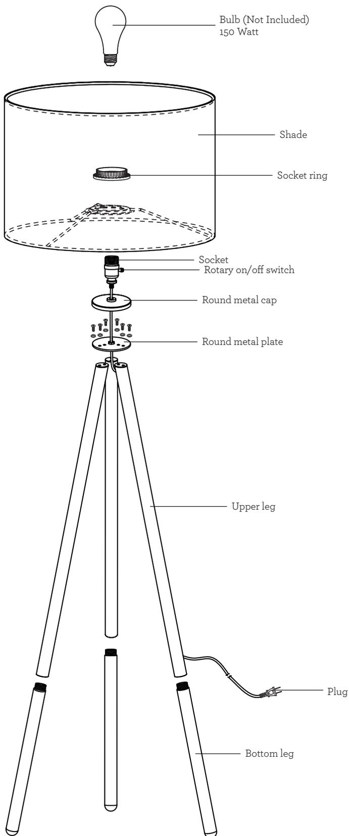
1. Assemble the round metal plate and upper leg with two screws and two washers then screw the bottom leg into the upper leg. Do the same to other two legs.
