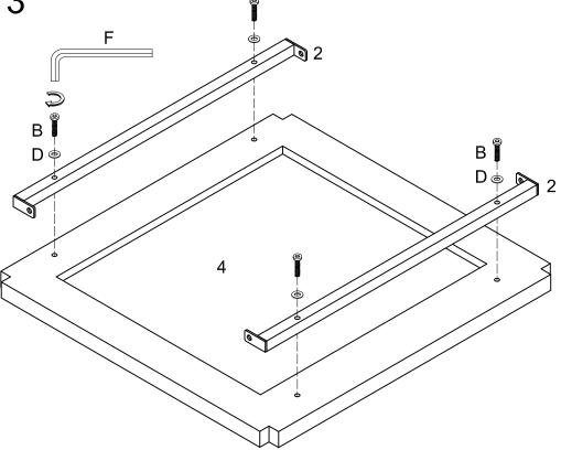
Attach part (2) to part (4) using bolts (B) and washers (D) as shown.
