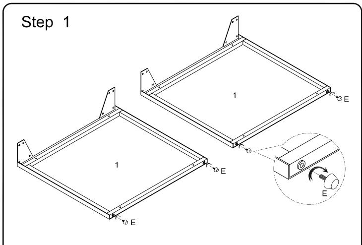
Screw foot pads (E) into frames (1) as shown in the diagram.
