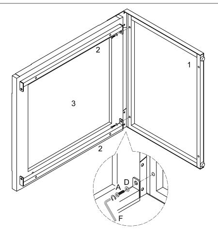
Join top panel (3) to part (1) using bolts (A) and washers (D).
