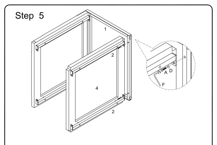
Join lower panel (4) to part (1) using bolts (A) and washers (D).
