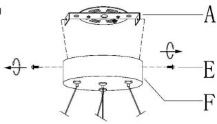
4 » Attach mounting plate (A) to the outlet box with mounting screws (D).
