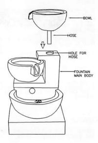
ATTACH PUMP TO THE HOSE FROM ACCESS PANEL ON REAR OF FOUNTAIN MAIN BODY. PLACE LED LIGHT ON FRONT RESERVOIR, FEED LIGHT CABLE THROUGH HOLE IN FRONT RESERVOIR, EXIT OUT FROM REAR ACCESS PANEL, READY FOR CONNECTION TO SOLAR PANEL.
