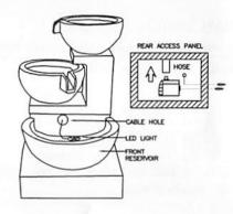
FILL RESERVOIR WITH APPROPRIATE AMOUNT OF WATER TO FULLY SUBMERSE THE PUMP.
