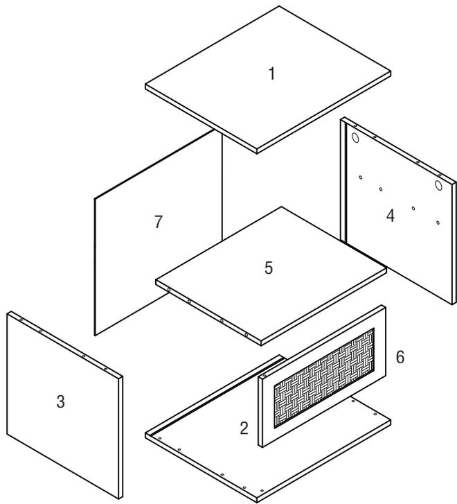
**1** Attach piece 3 & 4 to piece 5 using wooden dowels (C), cam dowels (A) and cam locks (B).
