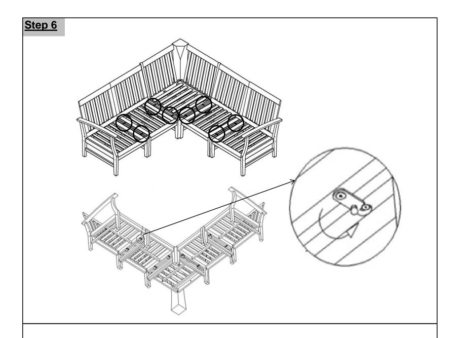
Note: This is optional step in case we want to connect all chairs in a set together and should be done before placing cushion With assistance from your adult partners, up side down the chairs and using pre-fixed clip to connect the chairs together.
