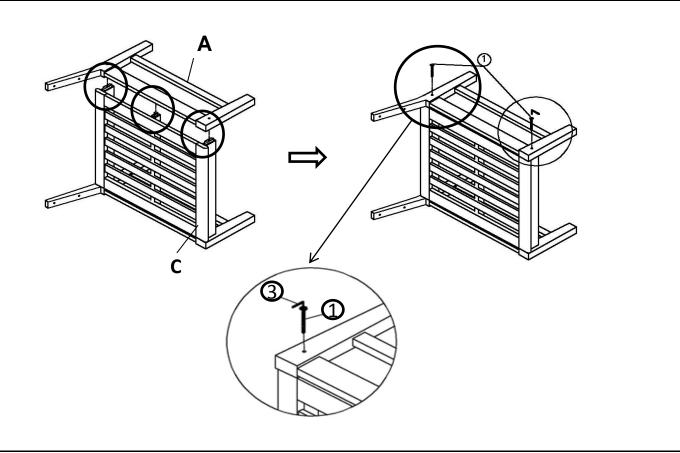
Attach mortise of Left Leg Panel With Pre-installed Levellers (B) to tenon of the Seat Panel (C) Secure by using Screw (1) with Allen Wrench(3).
