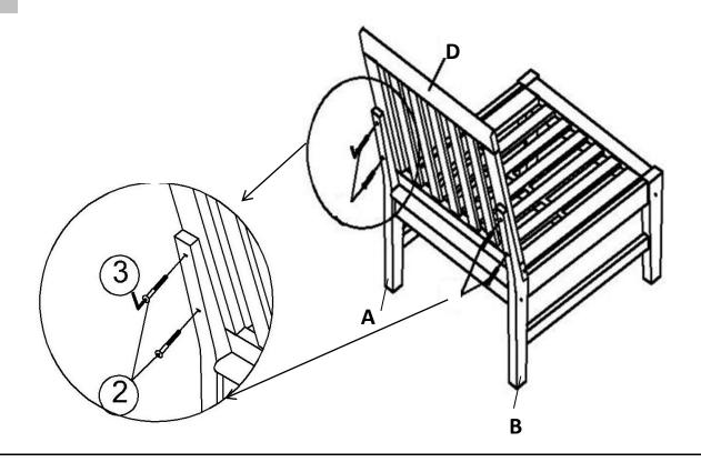
With assistance from your adult partners, turn the Chair right side up Attach Backrest Panel (D) to Right Leg Panel With Pre-installed Levellers (A) and Left Leg Panel With Pre-installed Levellers (B) by using Bolts (2) with Allen Wrench(3).
