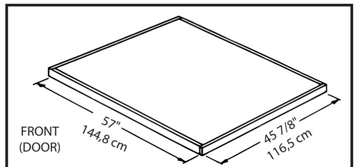
Note: Finished Slab dimensions, with lumber removed.
