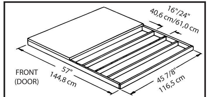
Note: Platform/Slab will extend 9/16" (1,4 cm) beyond floor frame on all four sides. Seal this 9/16" (1,4 cm) of wood with a roofing cement (not included), or bevel this 9/16" (1,4 cm) of concrete when pouring, for good water drainage.
