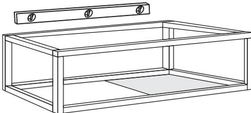
5. Set the basin on top of the frame, checking the location of the p-trap and drain. Remove basin from frame. Apply a thin bead of silicone adhesive around the top of the frame. Place the basin onto the frame and apply another thin bead of silicone to the edge of the basin. Remove excess silicone with a wet cloth.
