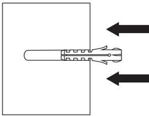
3. Place the frame up against the wall, be sure to align the anchors in the wall with the frame's mounting holes. Screw a metal screw into each anchor.
