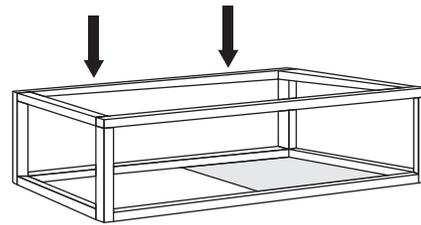
4. Ensure the frame is secure and level. Tighten if necessary- be sure not to overtighten.
