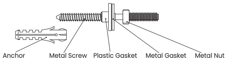
1. Measure the distance between the center of each mounting hole on the back of the frame. Use this measurement to draw 2 marks onto the wall in the desired mounting location. Use a level to make sure the marks are level with the floor. Drill 2 holes according to the marks using a 14 mm masonry drill bit to a depth of 75 mm.
