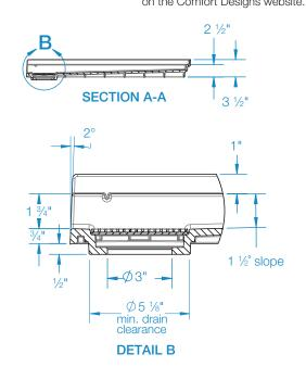
$FEATURES \ \ \, \text{Dimensional Tolerance} \,\, \pm \,\, \text{\%"}. \, \text{Dimensions needed for site preparation should be measured from the unit. Comfort Designs assumes no responsibility for preparatory work.}$
