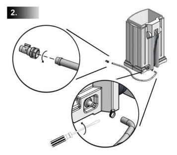
Attach the shut-off valve (part 7) to the threaded end of the garden hose (part 4). Next, attach the garden hose (part 4) to the rain barrel drain connector using the small clamp (part 5) to secure the hose in place. Tighten
