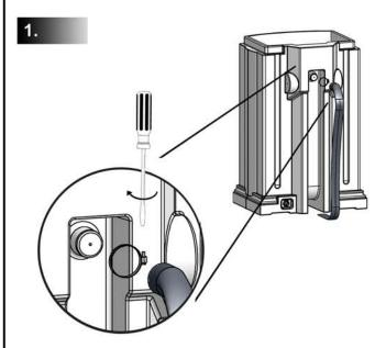
Attach the overflow hose (part 3) to the rain barrel overflow connector using the large clamp (part 6) to secure the hose in place. Tighten clamp with a slotted screw driver.
