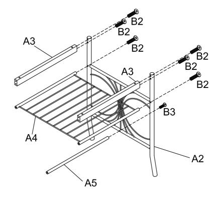
Assemble Connect Bars A3&A5 to Side Frame A2 using Bolts B2&B3. Note: Please do not tighten all bolts until Step 3.
