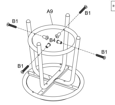
Attach Bottom Frame A9 to Legs A7&A8 using Bolts B1 with washers. Note:Please do not tighten Bolts B1 until Step 5.
