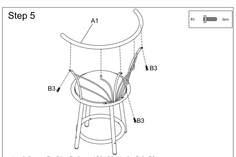
Attach Connect Bar B1 to Backrests A2&A3&A4 using Bolts B3. Note:Please place the chair to the floor to check if it is stable before tighten all bolts in 100%.
