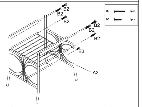
Assemble the other Side Frame A2 to Connect Bars A3&A5 using Bolts B2&B3. Note: Please do not tighten all bolts until Step 3.
