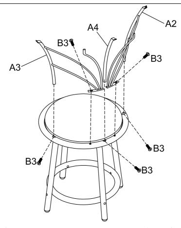
Attach Backrests A2&A3&A4 to Seat Frame A6 using Bolts B3. Note:Please do not tighten Bolts B3 until Step 5.
