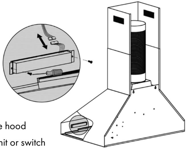
**NOTE:** Never work on or clean the range hood while power is ON. Always unplug the unit or switch the electrical breaker to the off position.
