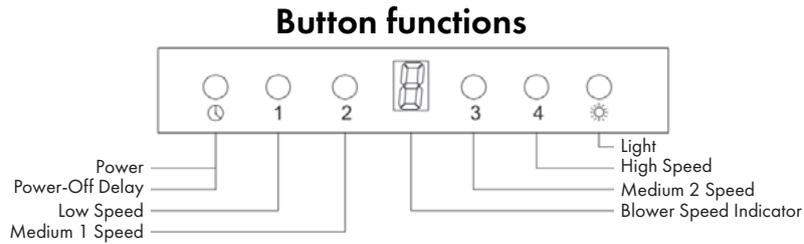
**Power:** Turn ON/OFF the range hood and activate power-off delay timer.
