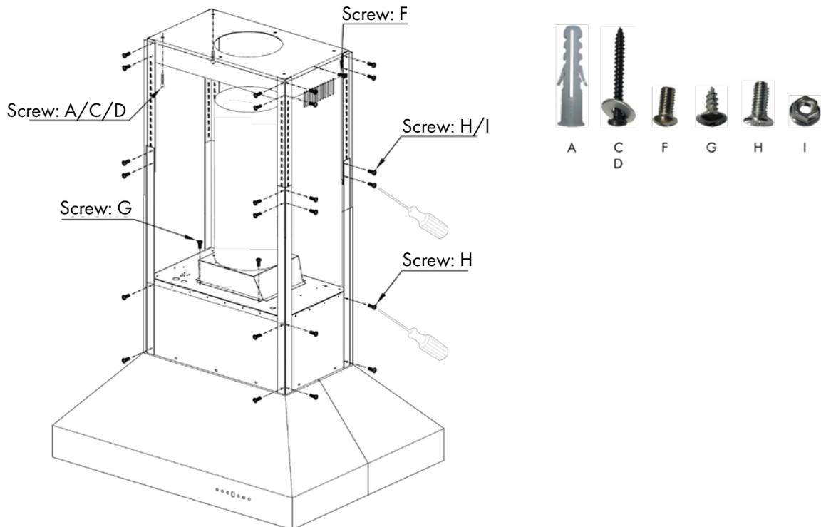
**NOTE:** Island range hoods with single motors will come with a square to 6" round transition piece and will include a back draft damper. The ducting with these range hoods is 6". Dual motor island hoods will come with a square to 8" round transition piece and in some instances are fitted with a built-in damper. For existing installations that may already have an external damper. Please consult an HVAC or installation professional for advice to comply with local regulations.
