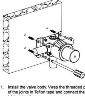
Install the valve body. Wrap the threaded portion of the joints in Teflon tape and connect the water inlet and outlet.
