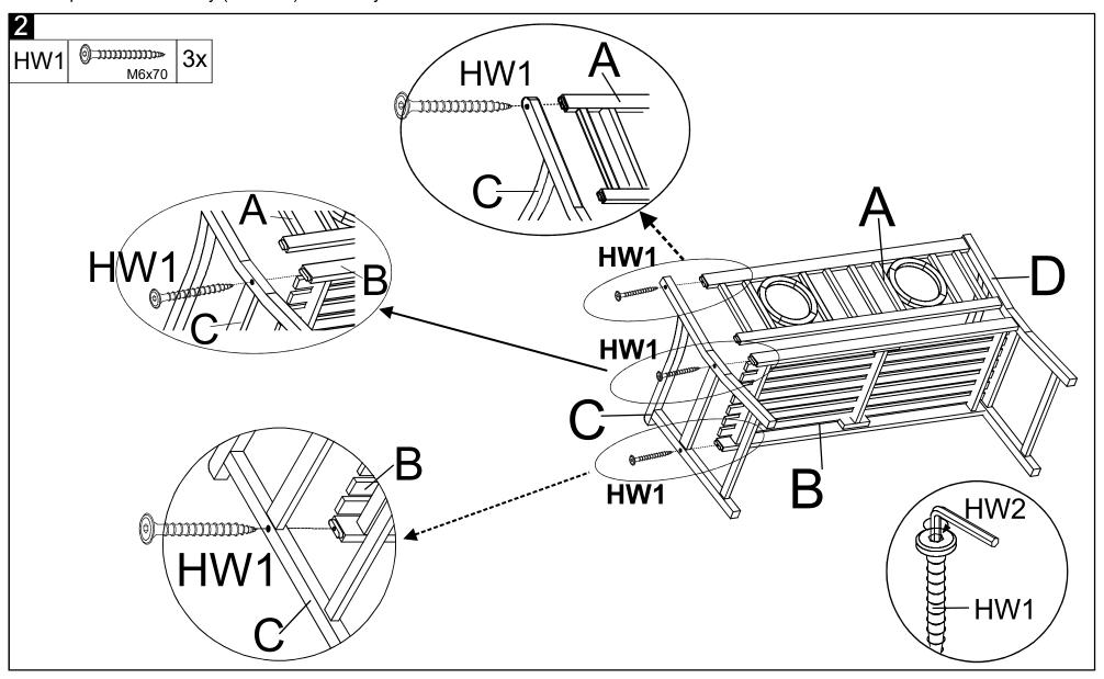
Step 2: Attach the Left side (C) to the Back (A) and the Seat (B) as shown in the picture . Using the Allen screw (HW1) to fix the Back (A), Seat (B) by the Allen key (HW2).
