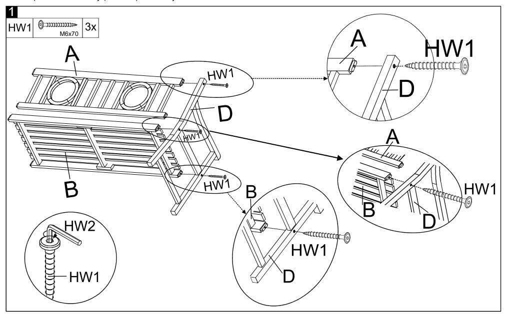
Step 1: Attach the Right side (D) to the Back (A) and the Seat (B) as shown in the picture . Using the Allen screw (HW1) to fix the Back (A), Seat (B) by the Allen key (HW2).
