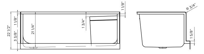
ATTENTION! Dimensions may vary by up to 3/8". It is highly recommended to pull all dimensions of actual model for installation and measuring purposes.
