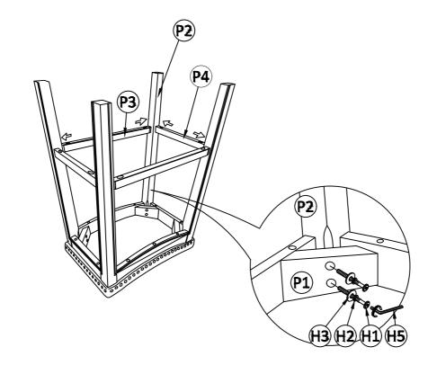
Step 5. Use Screw (H4) to fasten front stretcher (P3) and side stretchers (P4) to legs. Use screw driver to fix the screws. Tighten all bolts with allen key.
