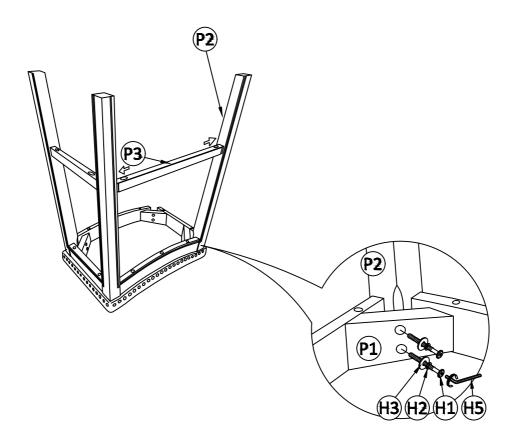
Step 4. Insert one of side stretcher (P4) and one front stretcher (P3) into hole on leg (P2). Loosely attach other leg (P2) to seat (P1), side stretcher (P4) and front stretcher (P3). Do not tighten bolts on this step.
