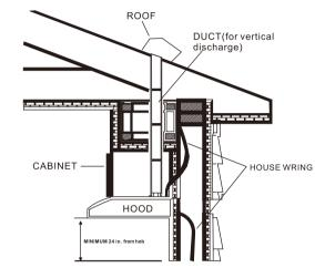
Determine whether the hood discharge vertically round (6in.) For vertically run ductwork between the hood location and the roof cap or wall cap. For the best result, use a minimum number of transitions and elbows.
