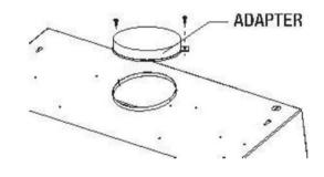
4. Measure the size of the outlet adapter relative to the cabinet and create an opening in the cabinet to let pass the outlet adapter and power cable. Make sure there is excess opening to accommodate electrical wires and hood exhaust. If you are installing the hood under the cabinet with a recessed bottom, it is advised to use a 4" wood fillers on both the sides.
