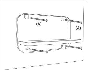
4. Secure the Folding Wall Shelf to the wall by the long screws(A).
