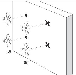
3.Insert the drywall anchors into the holes that have been drilled.
