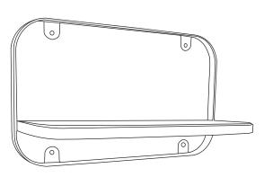
2. While holding the metal bracket against the wall, use a level to ensure that the metal bracket is level. Use a pencil to mark the holes on the wall.
