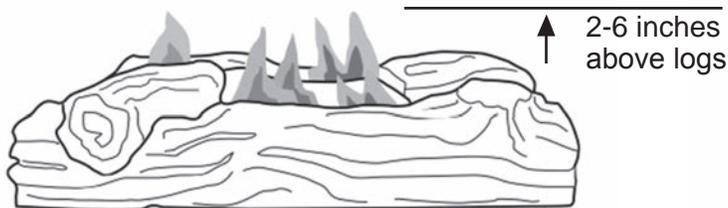
**Fig. 31 - Correct/Normal Flame Pattern with short flames**
