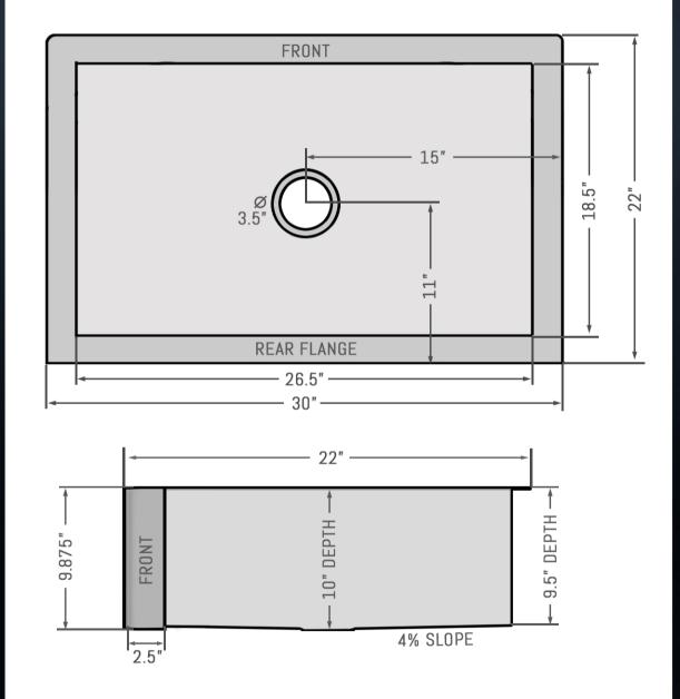
HANDMADE PRODUCT; MEASUREMENT TOLERANCES HELD TO +/- 2%
