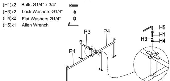
Step 2: Loosely attach Tray (P2) to Metal Leg A (P3) and Metal Legs B (P4) as shown below.
