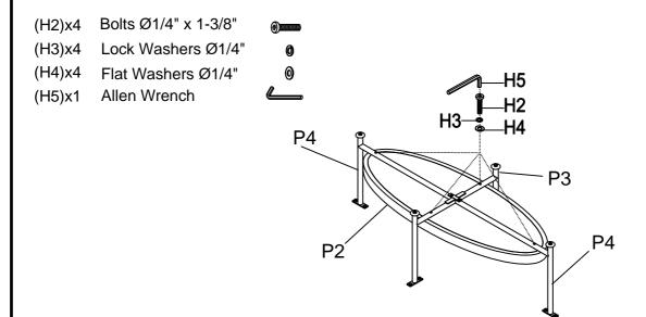
Step 3: Attach Metal Leg A (P3) and Metal Legs B (P4) to Table Top (P1) as shown below. Securely tighten all bolts by Allen Wrench (H5).
