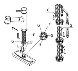
Insert spray hose (E) into small hole of base (D). Insert hot & cold waterlines (G) and supply hose (F), one by one, in large hole of base
