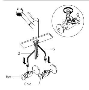
Thread hot & cold waterlines (G) onto angle stops. Tighten with adjustable wrench until snug. Turn on the angle stops and check for leaks.
