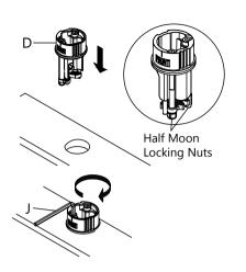
Insert base (D) into sink or countertop with "FR↑NT" facing forward. Tighten screws on base (D) with 4mm hex wrench (J) until base is secure on sink or countertop.
