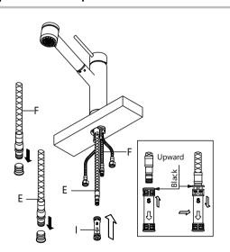
Attach Quick Connect (I) with black end onto spray hose (E) until you hear a click. Attach the other end onto the supply hose (F).
