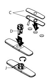
Place a bead of clear silicone sealant (not included) around the edge of the putty plate (C). Secure deck & putty plate (C) on sink or countertop. Insert base (J) into hole of deck & putty plate (C) with "FR1NT" facing forward. Tighten screws on base (D) with 4mm hex wrench (J) until base is secure on deck & putty plate (C).
