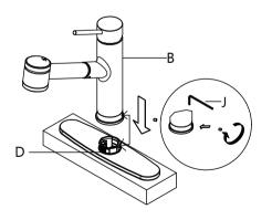
Align arrow on faucet body (B) with arrow on base (D). Attach faucet body (B) to base (D). Secure faucet body (B) by tightening the set screw with 2.5mm hex wrench (J).
