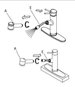
Remove spray head (A). Hold tip of spray hose (E). Turn faucet on for 1 minute to flush any debris. Reconnect spray head (A).
