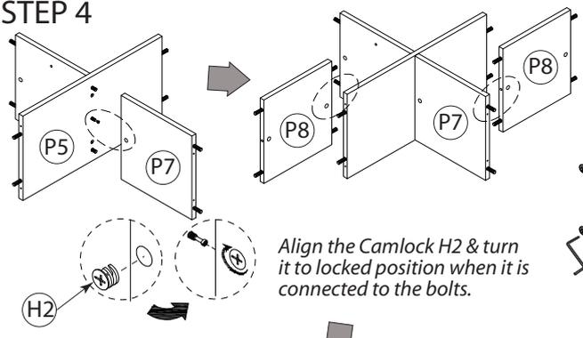
*Align the Camlock H2 & turn it to locked position when it is connected to the bolts.*
