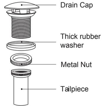
**Step 3:** From under the drain, insert the thick rubber washer, screw on and tighten the metal nut. Remove excess plumbers' putty.
