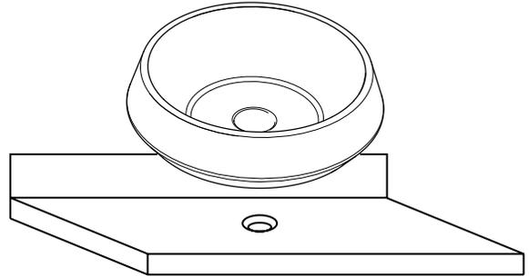
**Step 2:** Place a generous portion of plumbers' putty under drain cap and insert whole drain body inside the bowl and through the countertop.
