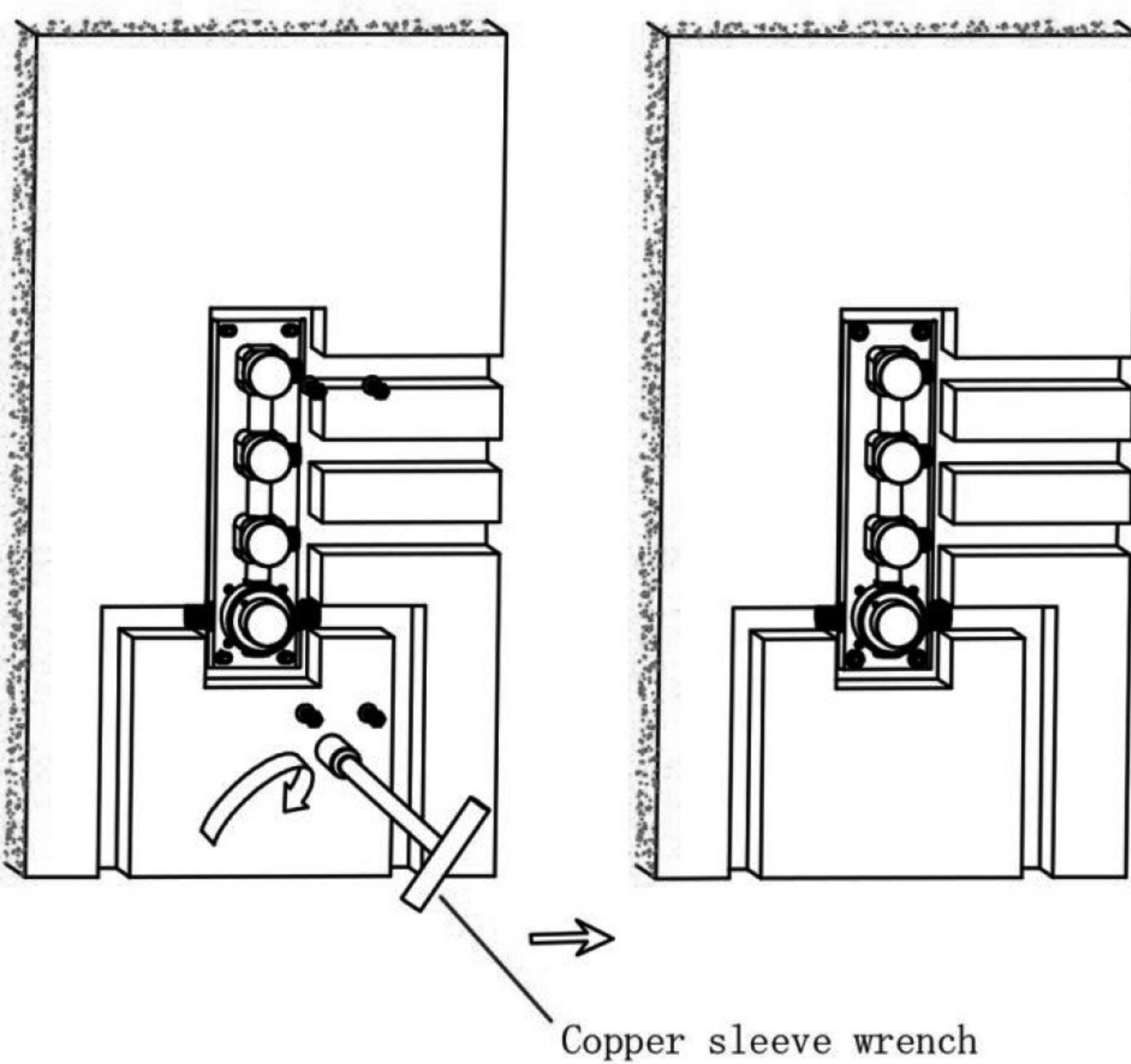
7. Take gaskets and spring gaskets onto the tapping screws. And then lock the nuts by copper sleeve wrench.
