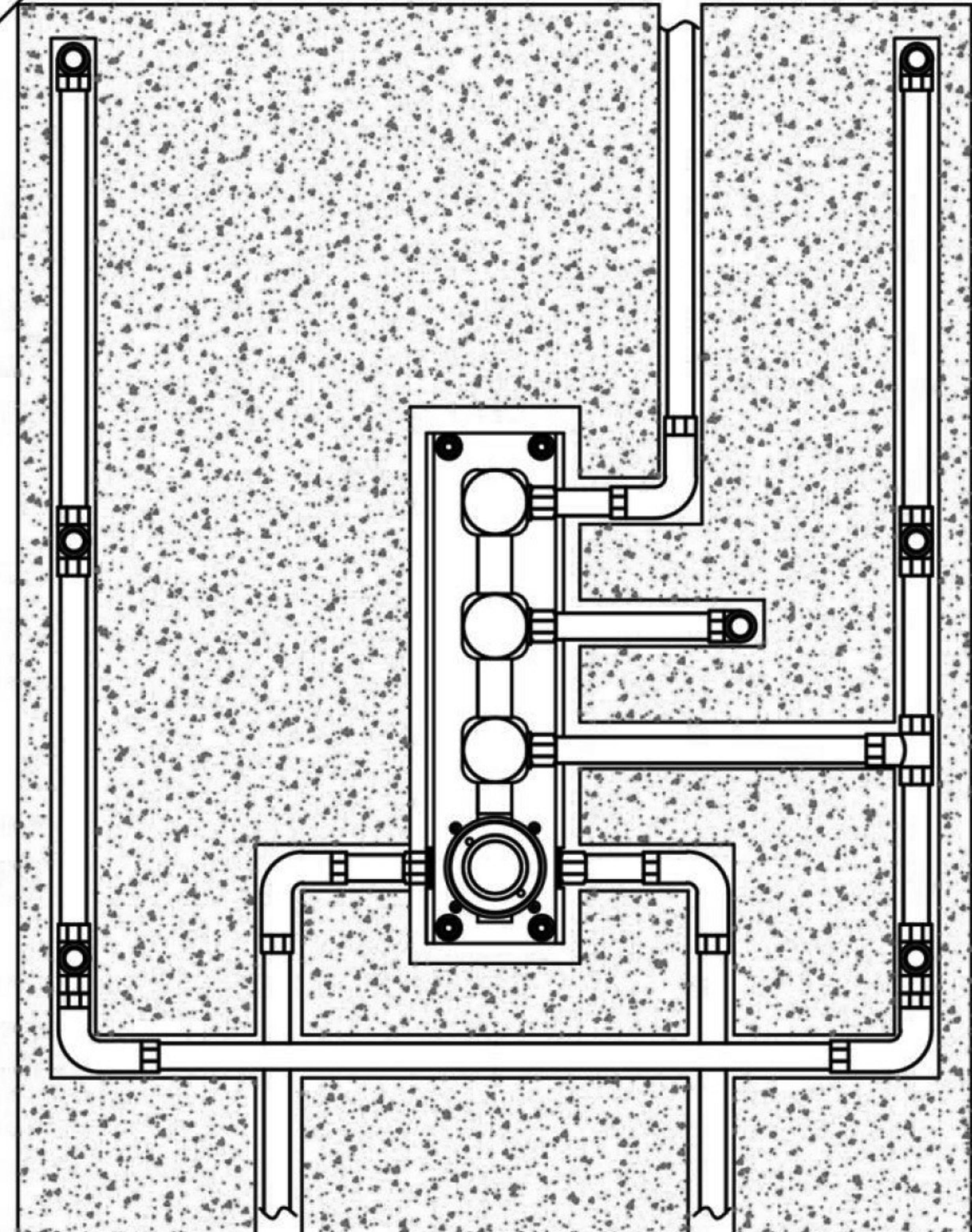
8. Connect hot & cold supply water pipes (not provided) and other water pipes. After that, open the water to test if all pipes have leakage or not. At last, seal the wall.
