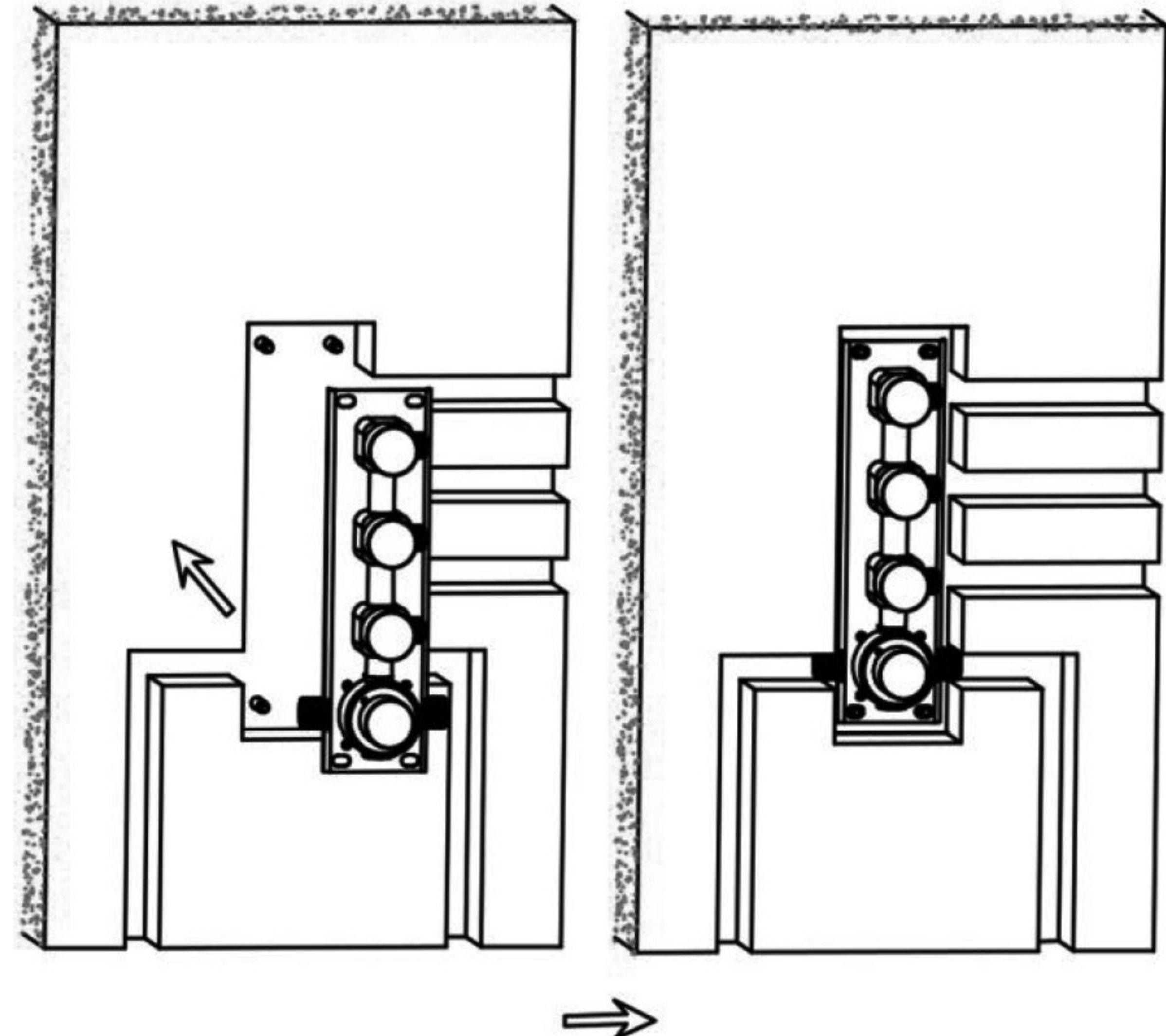
5. Place 4 tapping screws into the holes using hammer.
