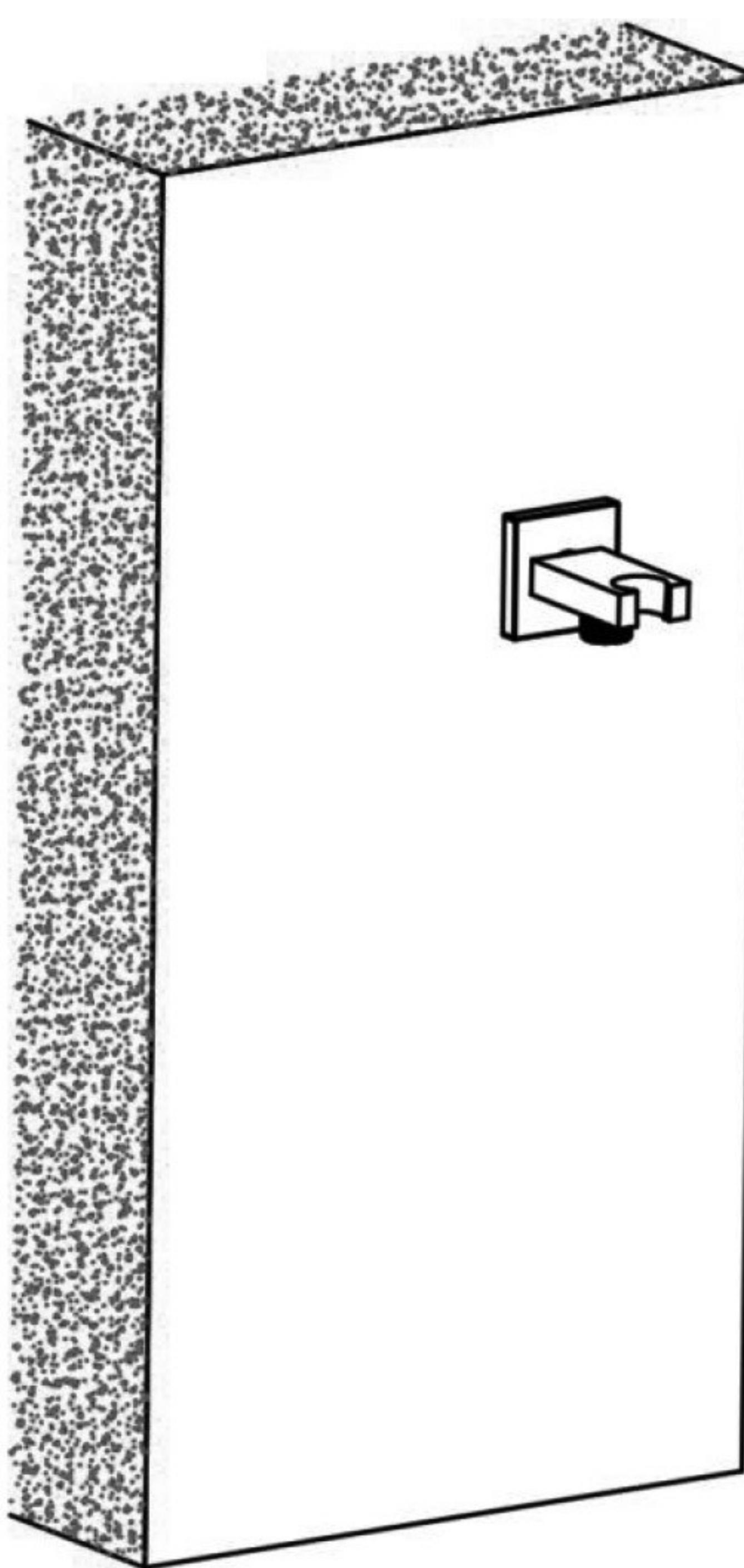
1. Wrap the 1/2 screw of holder with teflon tape to ensure a watertight seal
