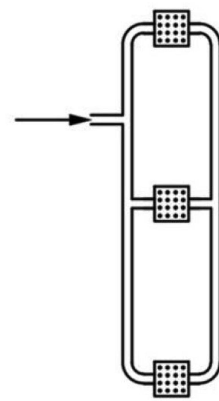
Multiple body jets will require installation in parallel using a pressure balancing loop (not included).
