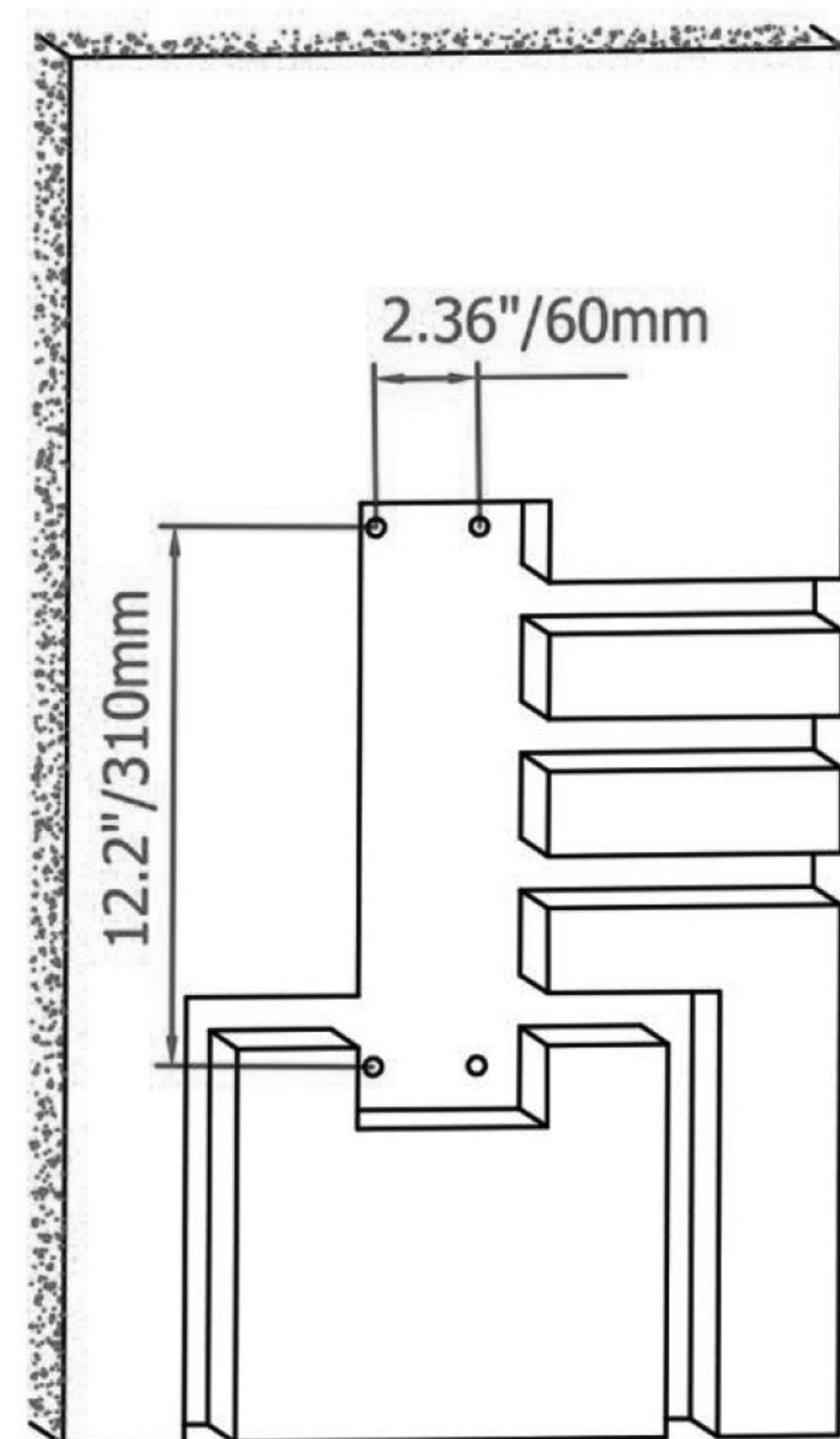
3. According to the actual size, get all pipe embedded mounts well ready.
