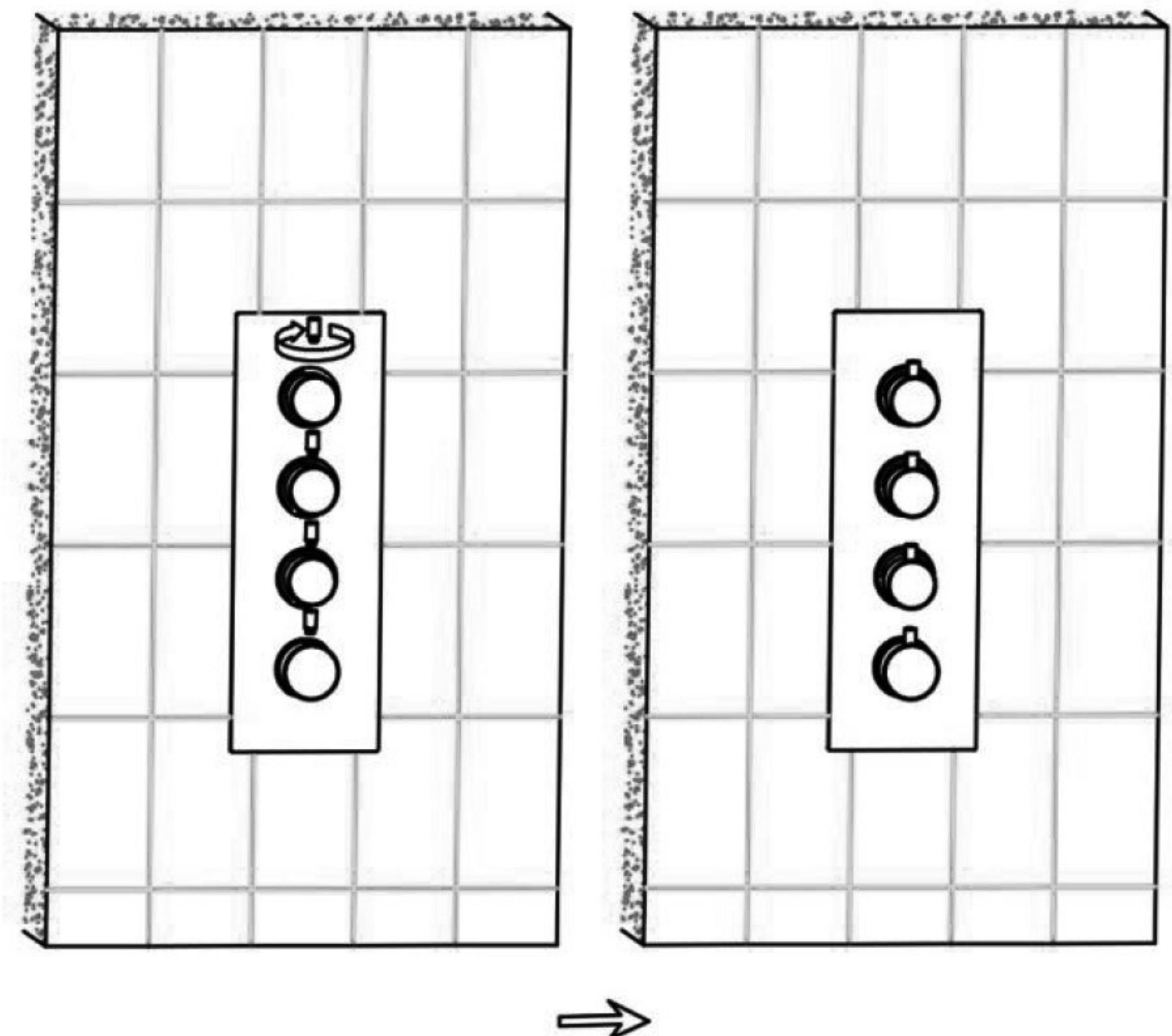
10. Screw the handles into the handwheels.
