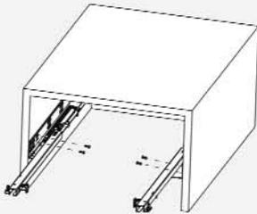
Pull out the drawer member of the slide from the cabinet, lay the drawer onto the slide.
