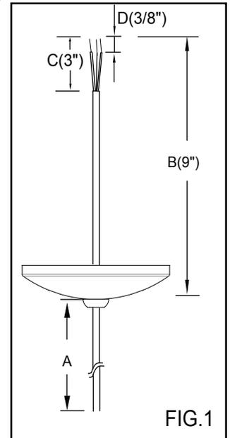
8. Pull the cord (A) down slightly until the strain relief touches the hex nut .Attach the canopy to the mounting strap by inserting two fixture mounting screws. then secure it with two ball nuts and two rubber pads.
