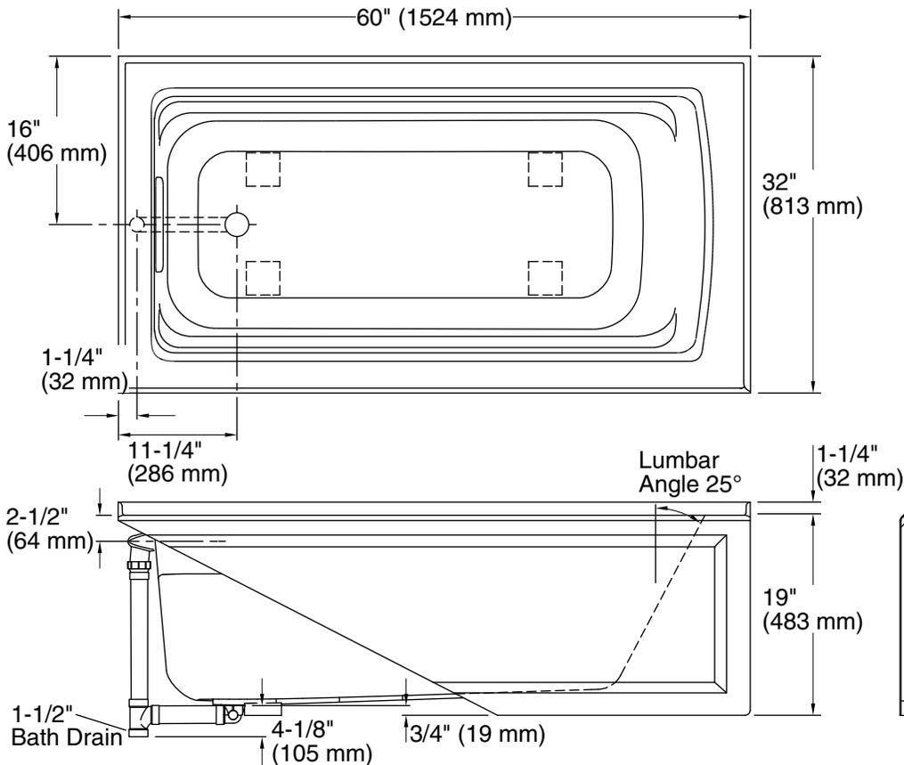
No change in measurements if connected with drain illustrated. (K-7272)
