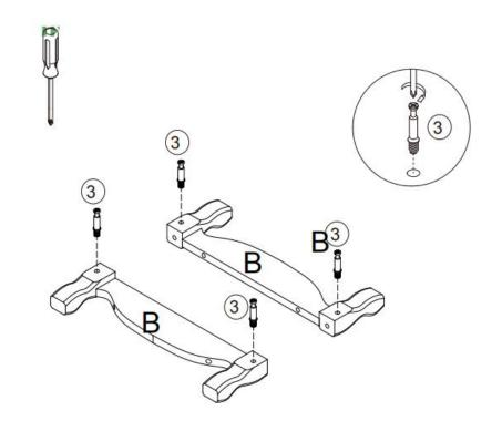
Be sure to check all packing material carefully for small parts, which may have come loose inside the carton during shipment. **STEP 1:** Use philips head screwdriver #5 to fasten cam bolt #3 on leg part B.
