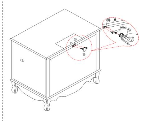
**STEP 4:**Insert screw #1 on part B&C,use philips head screwdriver #5 to fasten it.
