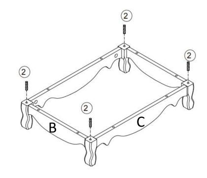
**STEP 2:**Use philips head screwdriver #5 to fasten cam lock #4 for secure part B & C.
