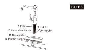
Position the faucet, deck plate and o-ring on the installation surface.
