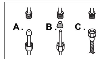
Connect to water supply lines with either:
