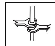
Tighten connection with two wrench to prevent
