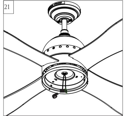
Isolate the quick connects with electrical tape.
