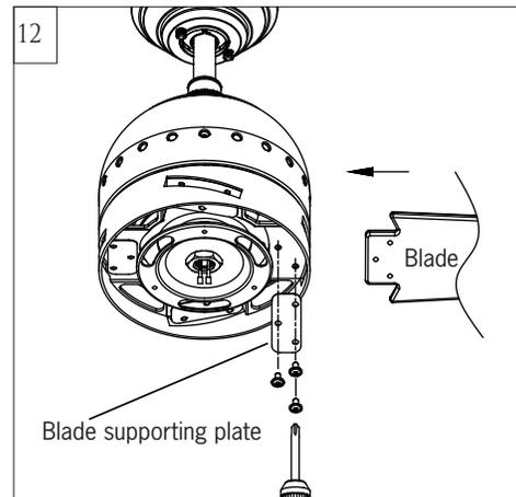
Insert blade into the slot on flywheel. Install blade with a blade supporting plate by the screws provided, aligning each of the holes as shown and tighten all screws securely. Repeat this process for remaining blades.
