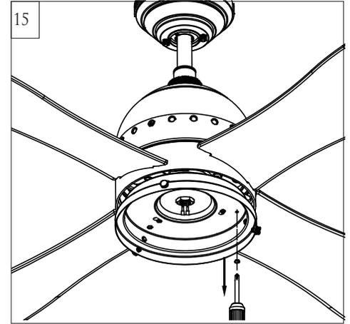
Loosen 2 and remove 1 preassembled screw from light pan. Save screw for later use.
