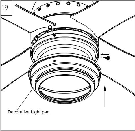
Align the holes on decorative light pan with the screw holes on light pan. Install it with the decorative set screws removed in the step 17.
