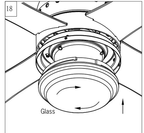
Attach glass by locating dimples in light pan with grooves on the glass and twist clockwise until tight.
