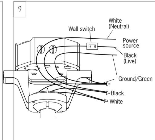
Make wiring connections using wire connectors provided as indicated above. Connect Black wire from fan to Black (Live) wire from house. Connect White wire from Fan to White (Neutral) wire from house. Connect all green grounded wires to Grounded wire from House. Make sure that no filaments are outside of the wire connectors.
