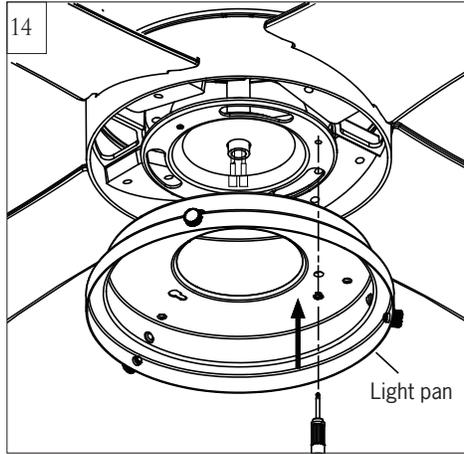
Place the lead wires from fan over the central hole of light pan. Aligning the keyhole slots on the light pan with the preassembled screws on the plate. Twist clockwise till lock. Reinstall the screw removed on installation step 13. Tighten all screws securely.
