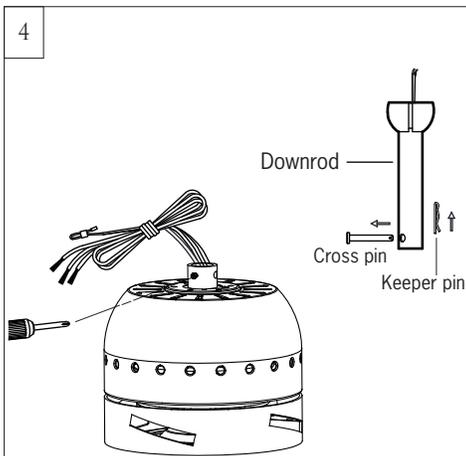
Partially loosen downrod set screws from yoke at top of motor assembly. Remove preassembled cross pin and keeper pin from downrod.
