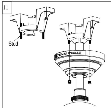
Lift Canopy allowing the 2 studs to protrude through the canopy. Install knurled nuts as shown. Tighten the knurled nuts securely. The canopy should adjust for any irregularity in the ceiling or Outlet box. Make sure the studs protruding from the bottom of the Mounting bracket are installed with threads all the way through the bracket.
