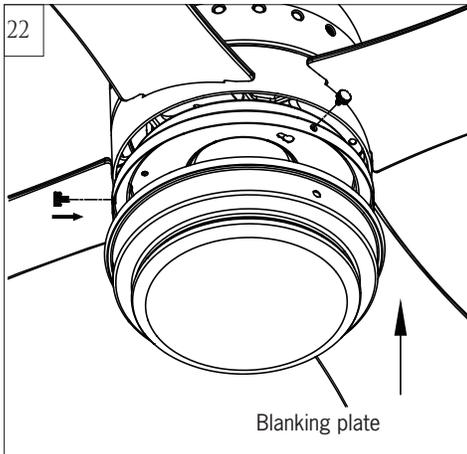
Install blanking plate. Align the holes on the blanking plate with the screw holes on light pan and reinstall the decorative setscrews removed in step 20.
