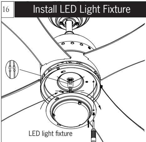
Connect white wire from fan to white wire from LED light fixture and then connect blue (or black) wire from light pan to black (or blue) wire from LED light fixture. Be sure plugs connection clasped together completely. Attach LED light fixture onto the light pan, aligning the keyhole slots on the LED light fixture with the preassembled screws on the light pan. Twist clockwise till lock. Reinstall the screw removed in the installation step 15. Tighten all screws securely.
