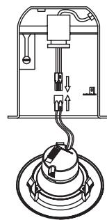
Connect the quick disconnect between the retrofit kit and the medium base umbilical socket.
