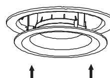
Push the LED retrofit trim into the recessed light fixture. Continue to push the LED trim until its outer edge is flush with the ceiling surface. **Turn on power.**
