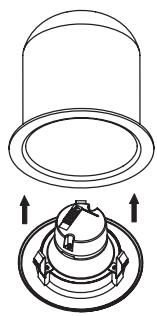
Slide the LED Downlight up into the recessed housing until the trim is flush with the ceiling.
