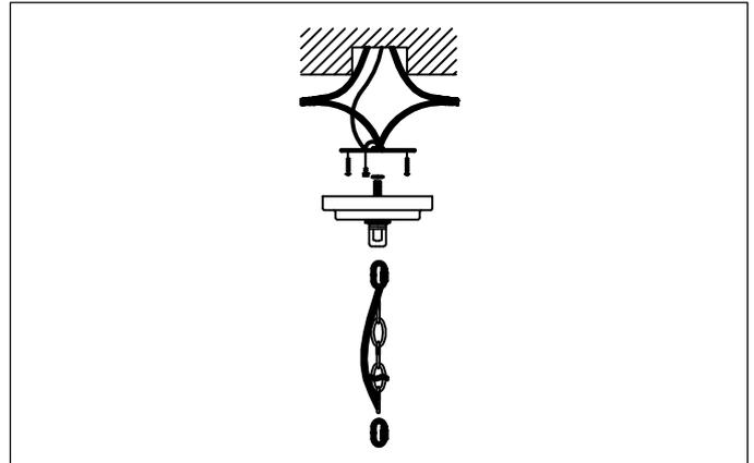
1. Attach rigid stem with top loop to the body of the fixture.
