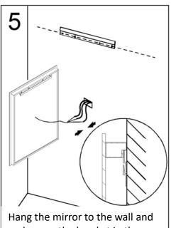
Hang the mirror to the wall and make sure the bracket in the back of the mirror lineup with the mounting bracket properly.
