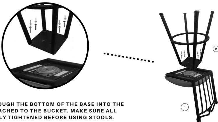
INSERT FOUR BOLTS THROUGH THE BOTTOM OF THE BASE INTO THE SWIVEL MECHANISM ATTACHED TO THE BUCKET. MAKE SURE ALL FOUR BOLTS ARE SECURELY TIGHTENED BEFORE USING STOOLS.
