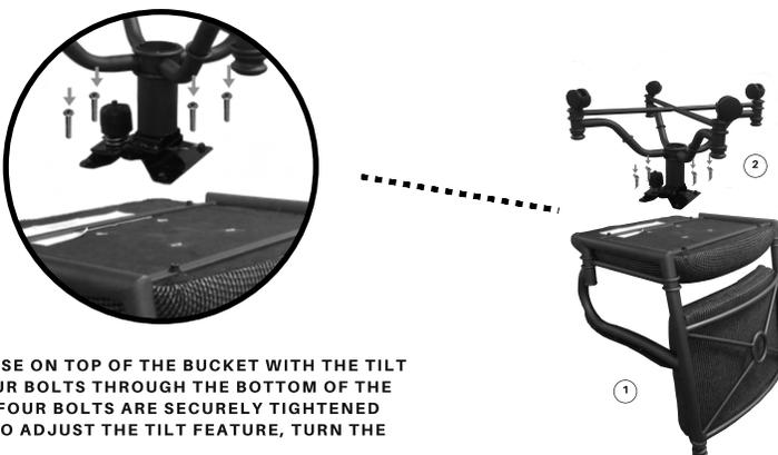
BEFORE INSERTING BOLTS, PLACE THE BASE ON TOP OF THE BUCKET WITH THE TILT ADJUSTER FACING FORWARD. INSERT FOUR BOLTS THROUGH THE BOTTOM OF THE BASE INTO THE BUCKET. MAKE SURE ALL FOUR BOLTS ARE SECURELY TIGHTENED BEFORE USING STOOLS/DINING CHAIRS. TO ADJUST THE TILT FEATURE, TURN THE TILT ADJUSTER FOR MORE OR LESS TILT.
