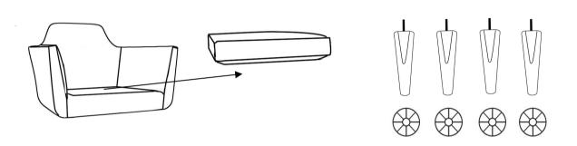
2. Screw in the feet (B) into the screw holes underneath the base using the plastic washers (C)
