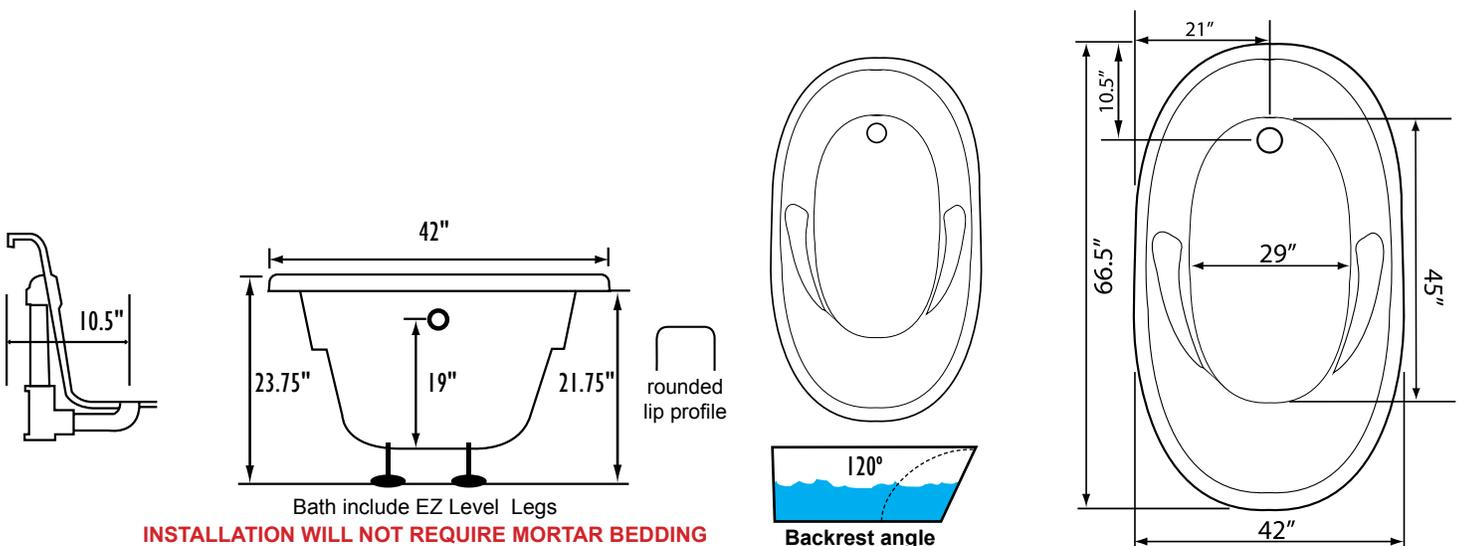
Some standard & most alternate pump locations may stickout past perimeter of the bath 1"-3". NOTE: Graphics may not be to scale. Specifications and features are subject to change without notice and are  $\pm .25"$ . All final measurements should be taken from tub on site. Access 18"x 18" or larger is required for each pump. Consult your contractor for installation requirements.
