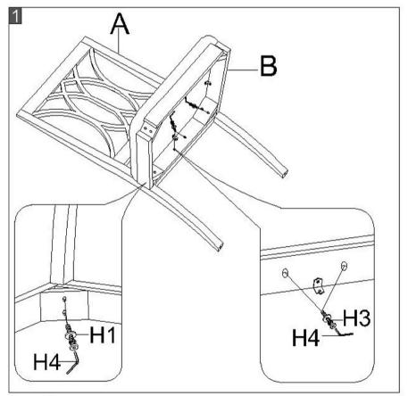
Step 1. Attach seat cushion (B) with chair back (A), Using Allen key (H4) to lock up Left / Right back legs by 4\*bolts (H1).
