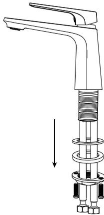
Remove the washer and mounting nut.
