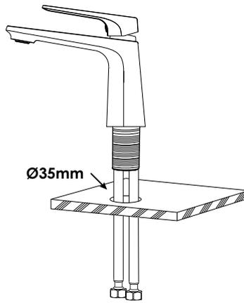
Ensure there is a Ø35mm through-hole on the counter. Position and insert faucet into faucet countertop hole.
