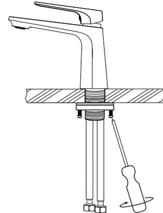
Tighten the mounting nut with the screws until faucet is firmly secure.
