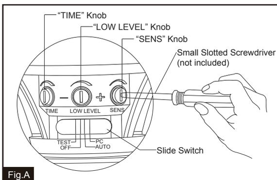
Step 1: Rotate the sensor lens from left side to right side to show the adjustable knobs and slide switch. (See Fig.1)
