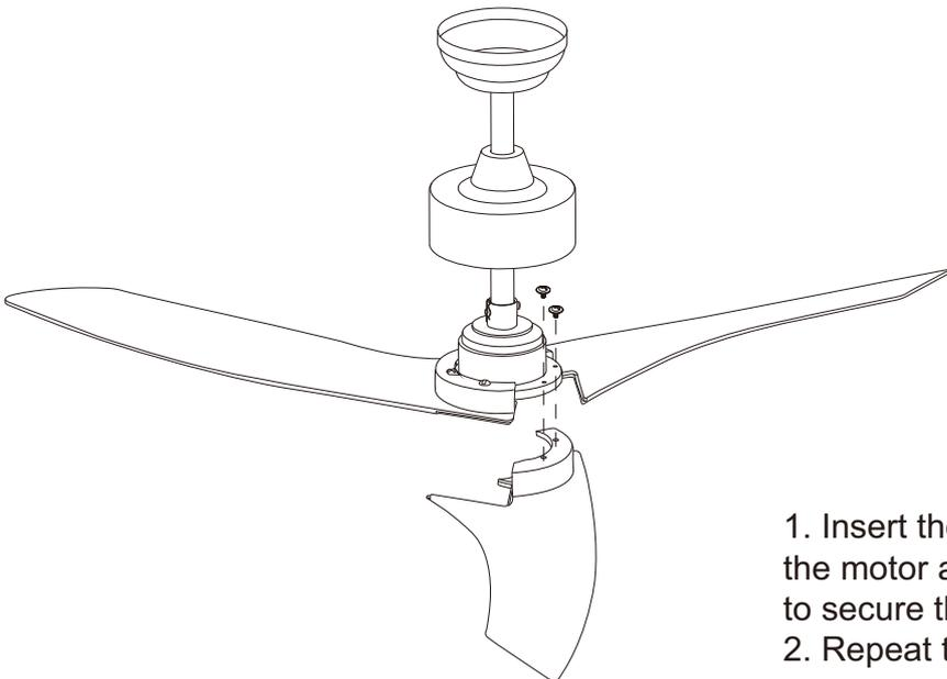
1. Insert the positioning column into the slot above the motor and tighten the preinstalled blade screws to secure the blade to the fan motor assembly.
