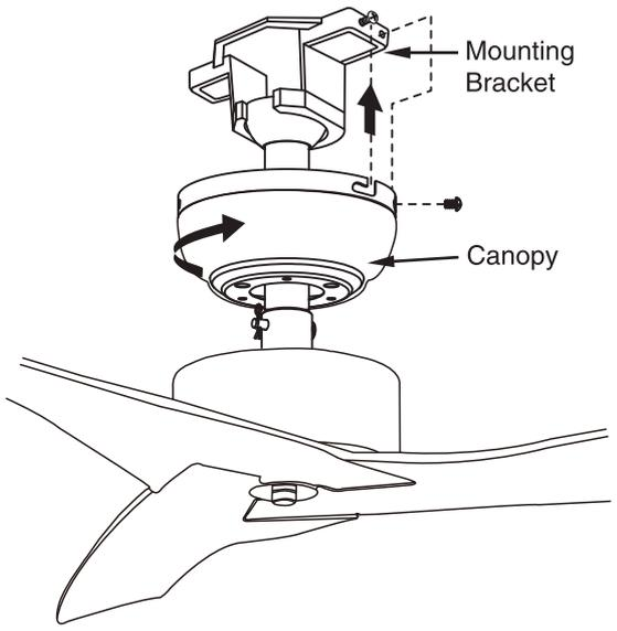
1. Notice the half ball on the end of the support rod is grooved down one side. This key way fits over the small keyway pin on the inside of the mounting bracket and keeps the ceiling fan from spinning on the mounting bracket.
