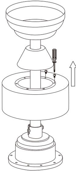
1. Remove the six screws on the shell of the fan motor to separate the shell from the motor.
