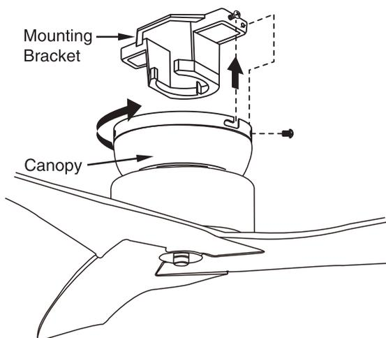
Slide the canopy up into place over the ceiling mounting bracket. Loosen up the canopy screws on the side of the canopy screws. Press the canopy against the mounting bracket and turn it clockwise. Tighten screws on the J Slots and install the two screws in the remaining holes.
