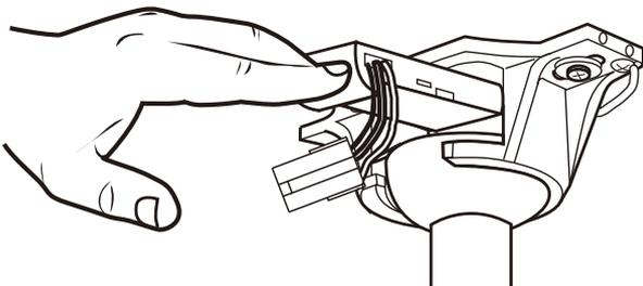
1. Carefully push the canopy to the bottom of the mounting bracket, make two sliding holes aligned to the two prominent screws on the mounting bracket, and then turn clockwise until tight.
