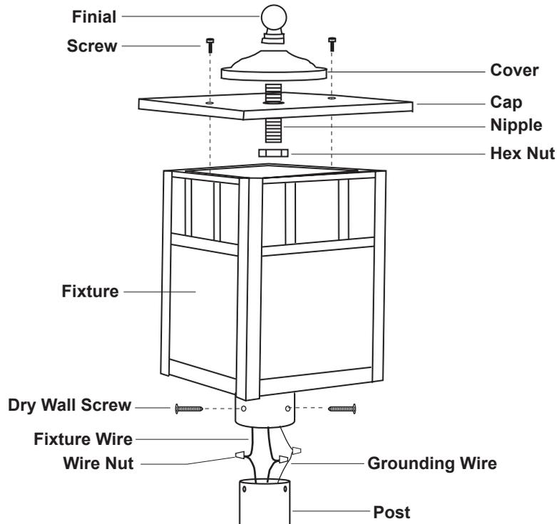
1. Pull out the outlet wires and grounding wire from the post. Make wire connections using the wire nuts:
