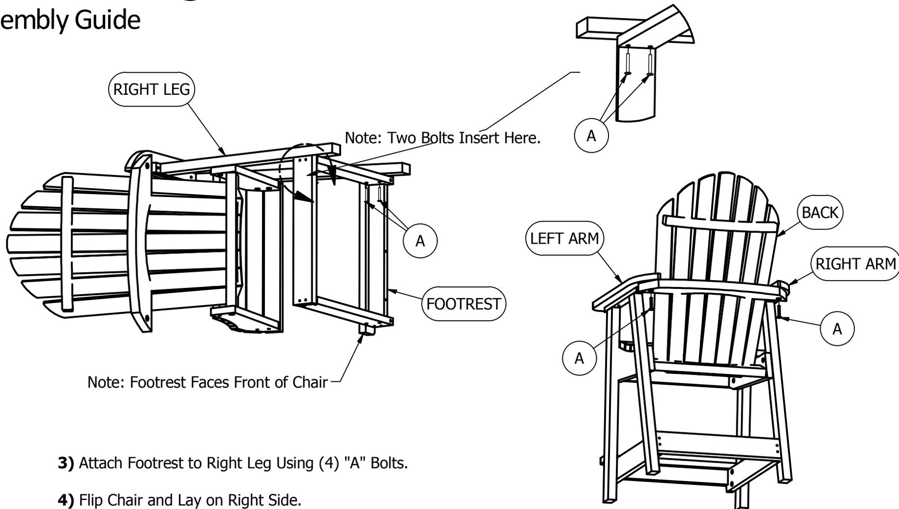
**3)** Attach Footrest to Right Leg Using (4) "A" Bolts.
