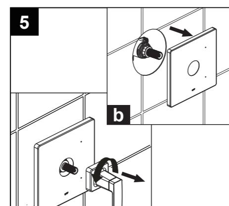
a Unscrew the handle assembly counter-clockwise from valve and remove the escutcheon.
