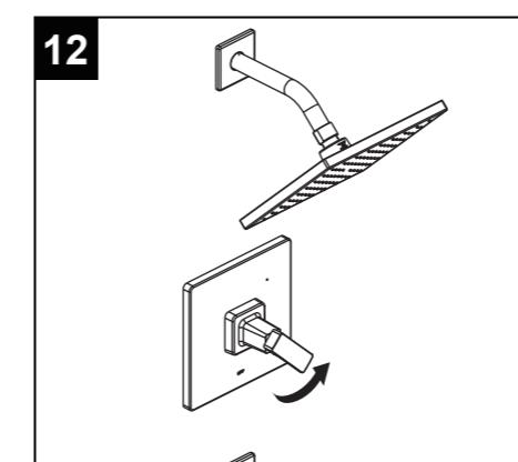
Turn on the handle and check the function of the spout.
