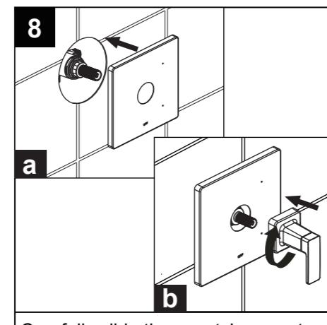
a Carefully slide the escutcheon onto the valve and place handle assembly on valve and rotate clockwise to secure escutcheon.
