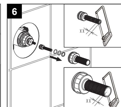
b Cut stem and nipple the amount noted in step #4. (Never cut the stem and nipple while still on the valve. This may damage the valve.)
