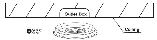
Align canopy cover (A) and outlet screws (B) with outlet box.
