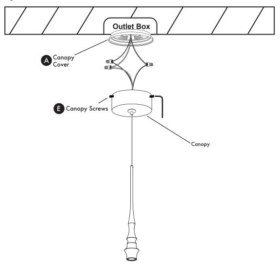
Attach canopy to canopy cover (A). Secure with canopy screws (E).
