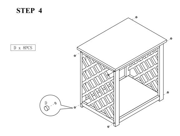
1. COVER HEX BOLT HOLE WITH WOOD PLUGS (D) AS SHOWN.
