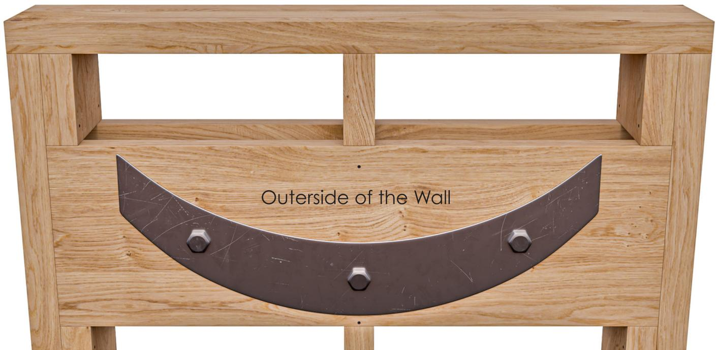
The ideal height of the metal plates is 19" from the finished floor to the center of the low center bolt, which would leave the tub hanging about 6" from the bottom of the tub to the floor and 4" from the bottom of the drain splash guard. You can go up to 2" lower or higher if desired.
